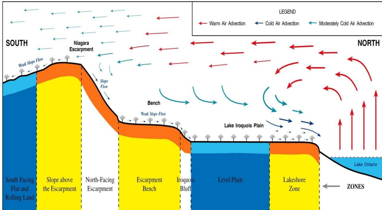
On clear, calm nights complex circulation systems develop over the Niagara region caused by the interaction of warmer air rising over the lake-surface and colder air lying over the land mass. As the warm air rises over the lake and moves inland, the cooler air from the land mass is drawn over the lake to replace the rising air, creating a closed circulation that can modify temperatures several kilometers inland.
